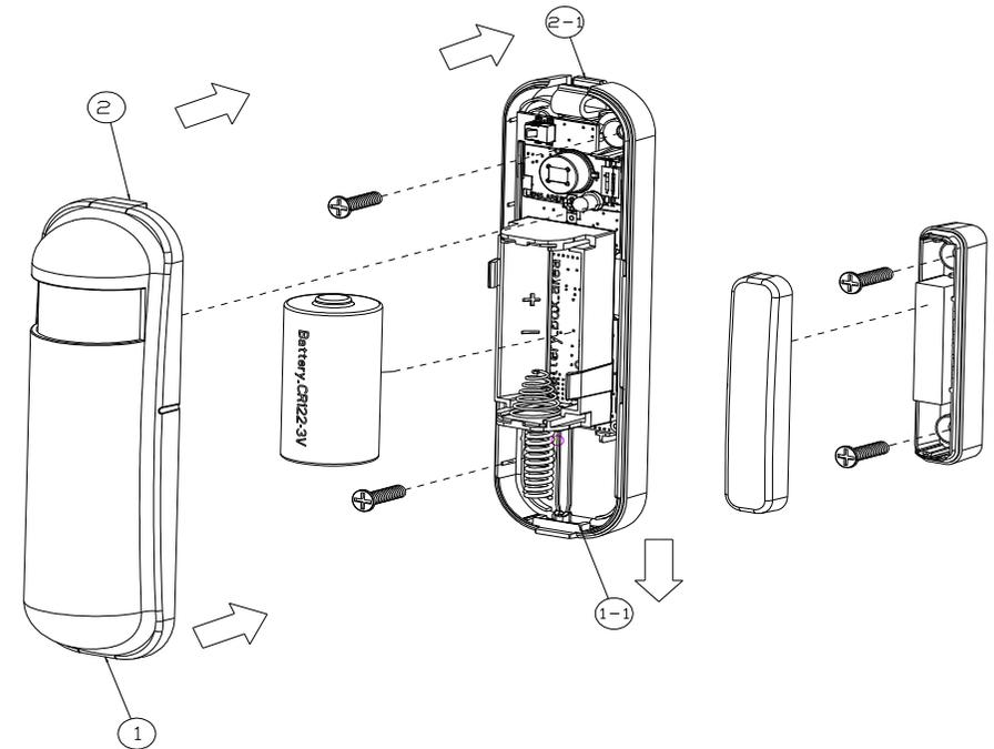
Replace the new battery and install the cover back.
